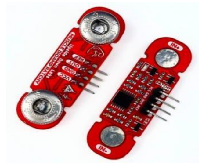
Figure 1. Muscle BioAmp Patchy Sensor
