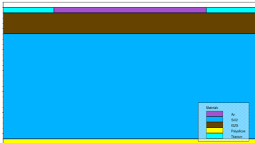
Fig: 3; Two-dimensional schematic representation of amorphous-IGZO TFTs structure used in this paper
