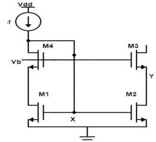
**Fig. 3** Wide swing cascode current mirror
