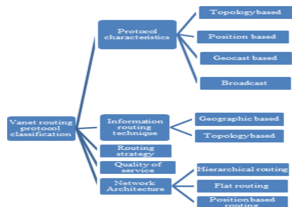
Fig. 5 Classification of VANET Routing Protocol
