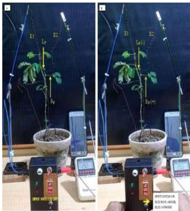
Fig. 7 A – Before Stimulation, B – After stimulation Left petiole (electrode E1) cathode, Right petiole (electrode E2) anode.
