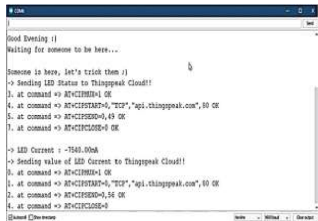
Fig. 9 The output of proposed system and LEDcurrent (in mA) showing and sending to ThingSpeak cloud
